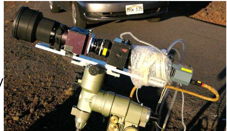
A filter imager used for observations of Jupiter's sodium nebula.
