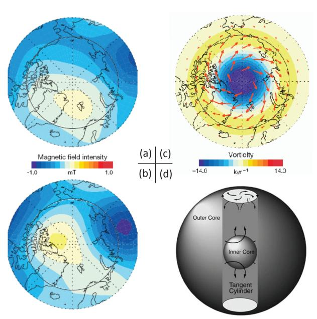
(a,b) Geomagnetic field at the outer core surface at epochs 1870 and 1990, northern hemisphere; (c) Inferred axisymmetric surface flow structure; (d) A thermal wind inside the tangent cylinder: upwelling near the spin axis, prograde above the inner core surface, retrograde below the outer core surface [Adapted from Olson & Aurnou, 1999]
