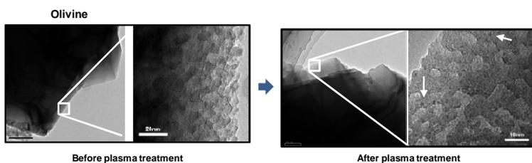
TEM images of untreated olivine powder and olivine powder after hydrogen plasma treatment. Although the surface of the untreated particle is angular shape, the surface is changed into round shape after plasma treatment. As shown by arrows, black spots with the size of about 1nm are seen in high resolution TEM image. This result suggests that the particles react with hydrogen plasma to cause the surface alteration.
