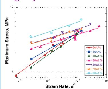
0-10wt.%:  $\sigma_{\max}$  does not depend on the silica content.
