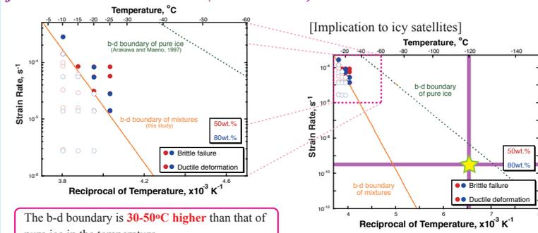
The b-d boundary is **30-50°C higher** than that of pure ice in the temperature.
