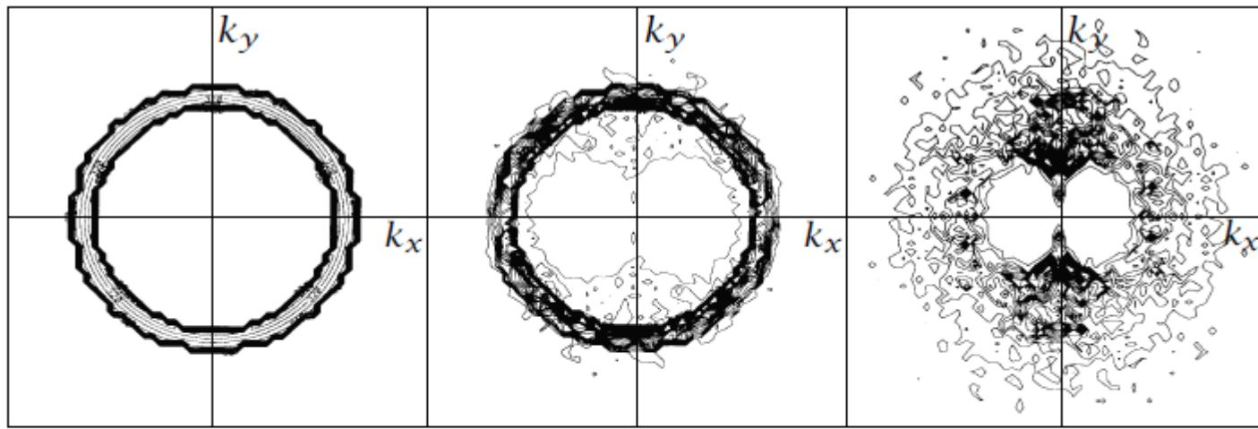
**Fig. 12.3** Evolution of the energy spectrum in a freely evolving two-dimensional simulation on the  $\beta$ -plane. The panels show contours of energy in wavenumber ( $k_x, k_y$ ) space at successive times. The initial spectrum is isotropic. The energy ‘implodes’, but its passage to large scales is impeded by the  $\beta$ -effect, and the second and third panels show the spectrum at later times, illustrating the dumbbell predicted by (12.14) and Fig. 12.2.<sup>2</sup>
