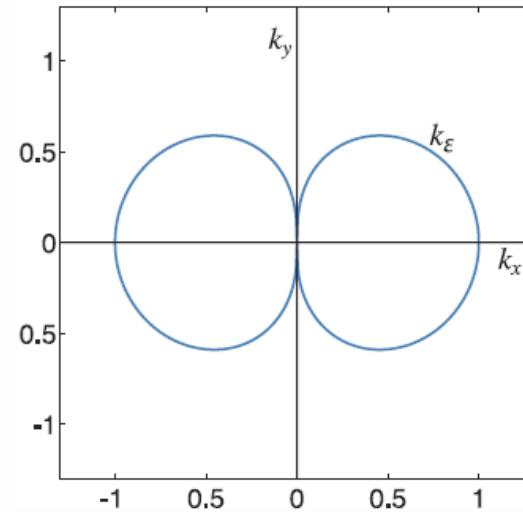
**Fig. 12.2** The anisotropic wave-turbulence boundary  $k_\epsilon$ , in wave-vector space calculated by equating the turbulent eddy transfer rate, proportional to  $k^{2/3}$  in a  $k^{-5/3}$  spectrum, to the Rossby wave frequency  $\beta k^x/k^2$ , as in (12.14). The wavenumbers are scaled such that  $\beta^3/\varepsilon = 1$ .
