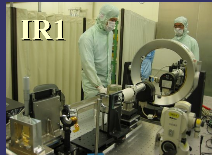
Photos of IR1 lens assembly tests (top: vibration test, bottom: optical performance test)
