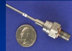
MEMS seismic event sensor Courtesy: Tom Pike
