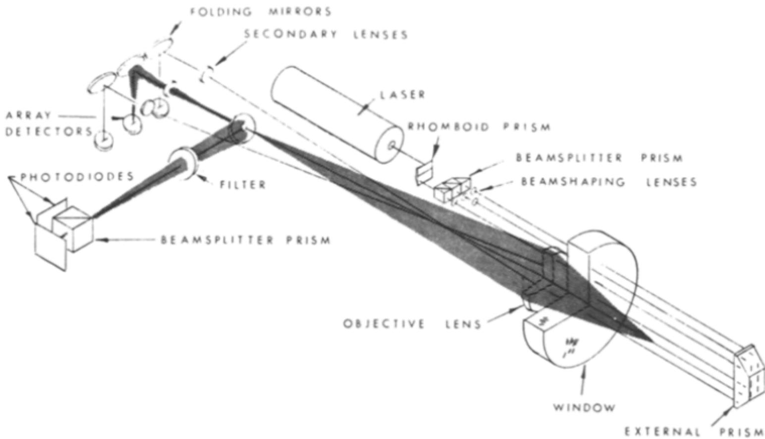
Fig. 11. (LCPS). LCPS optical diagram.
