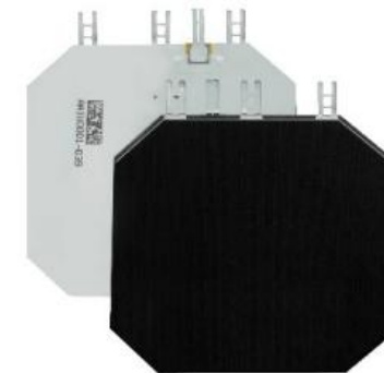
Cells shown with interconnects, coverglass, and bypass diode
