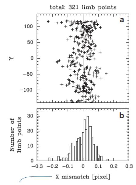
Displacement between each limb poin location and fitted ellipse
