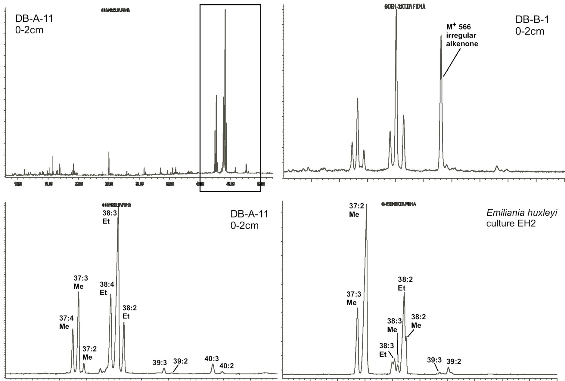
Fig. Gas chromatograms of ketone fractions in sediments of Dabusu Lake.
