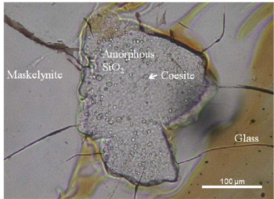
Figure 1. Optical microscopic image of coesite.
