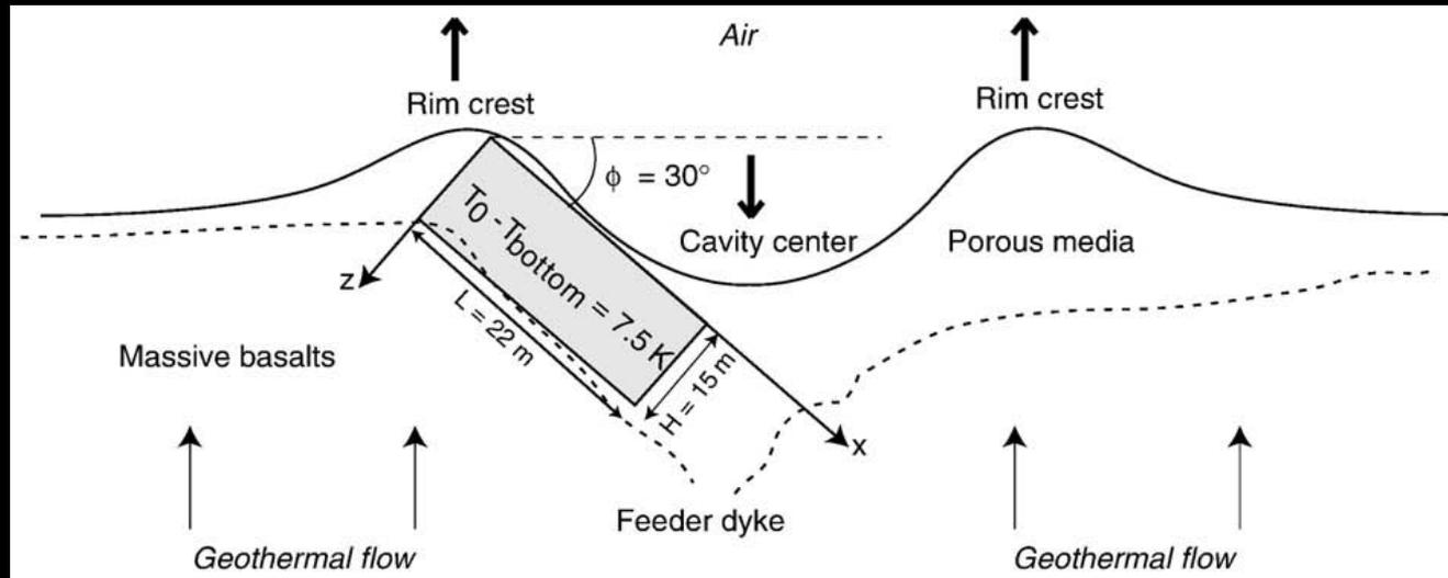
Representation of the box used for the air convection model.
