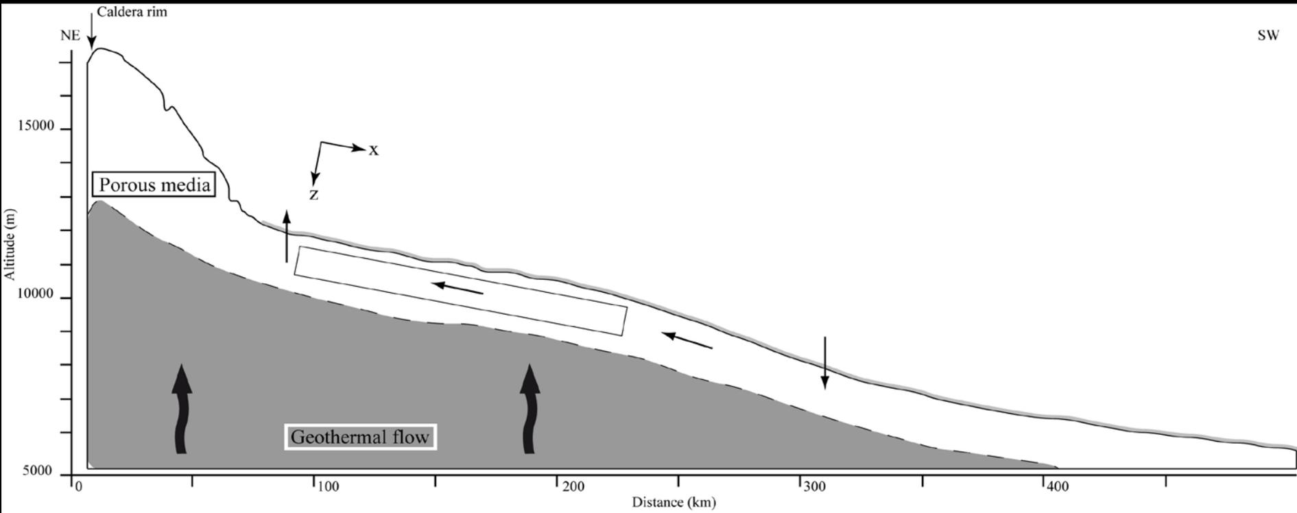
Representation of the box used for the air convection model.
