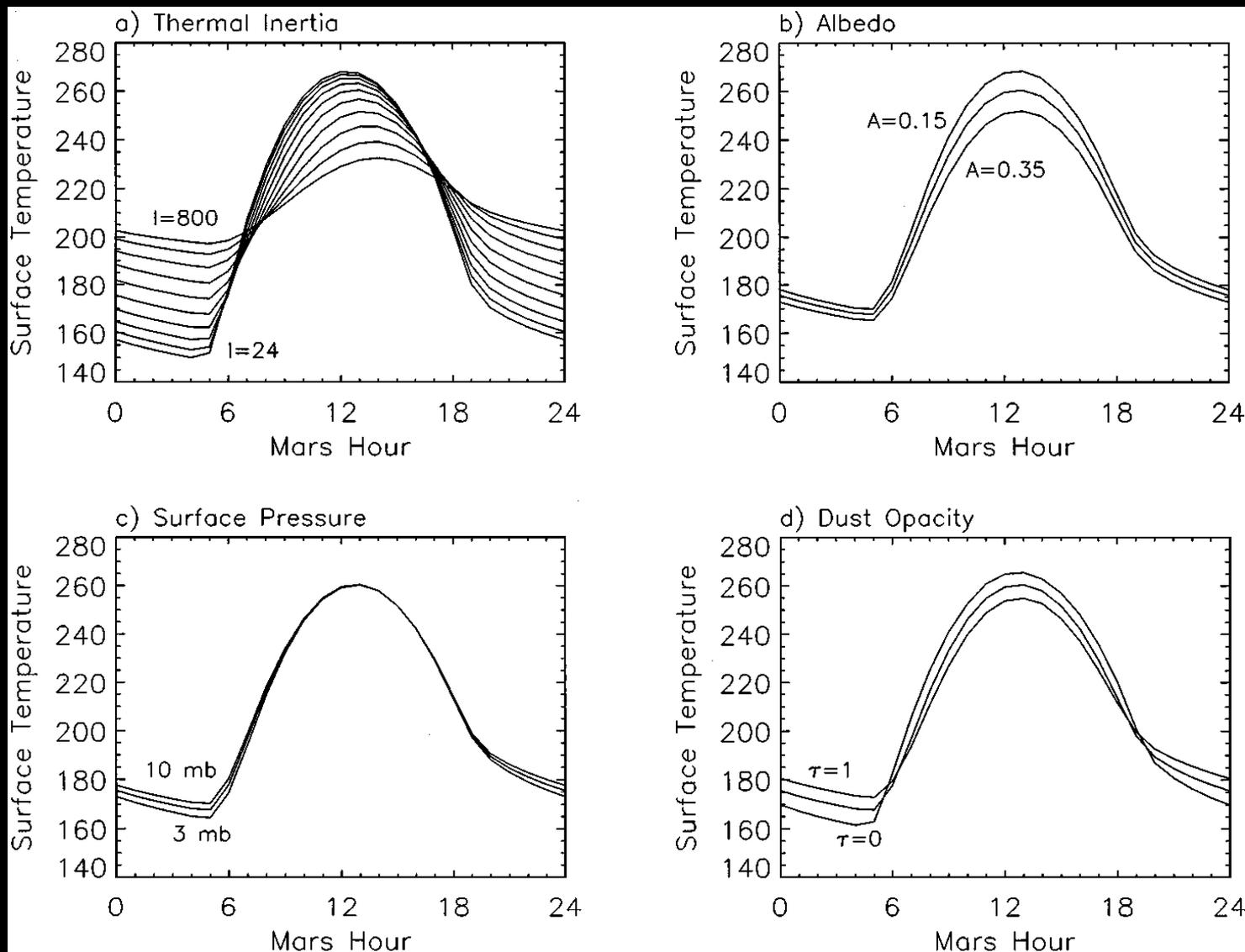
Influence of the thermal inertia, the albedo, the surface pressure and the dust opacity on the variation of diurnal surface temperature (Mellon et al, 2000)
