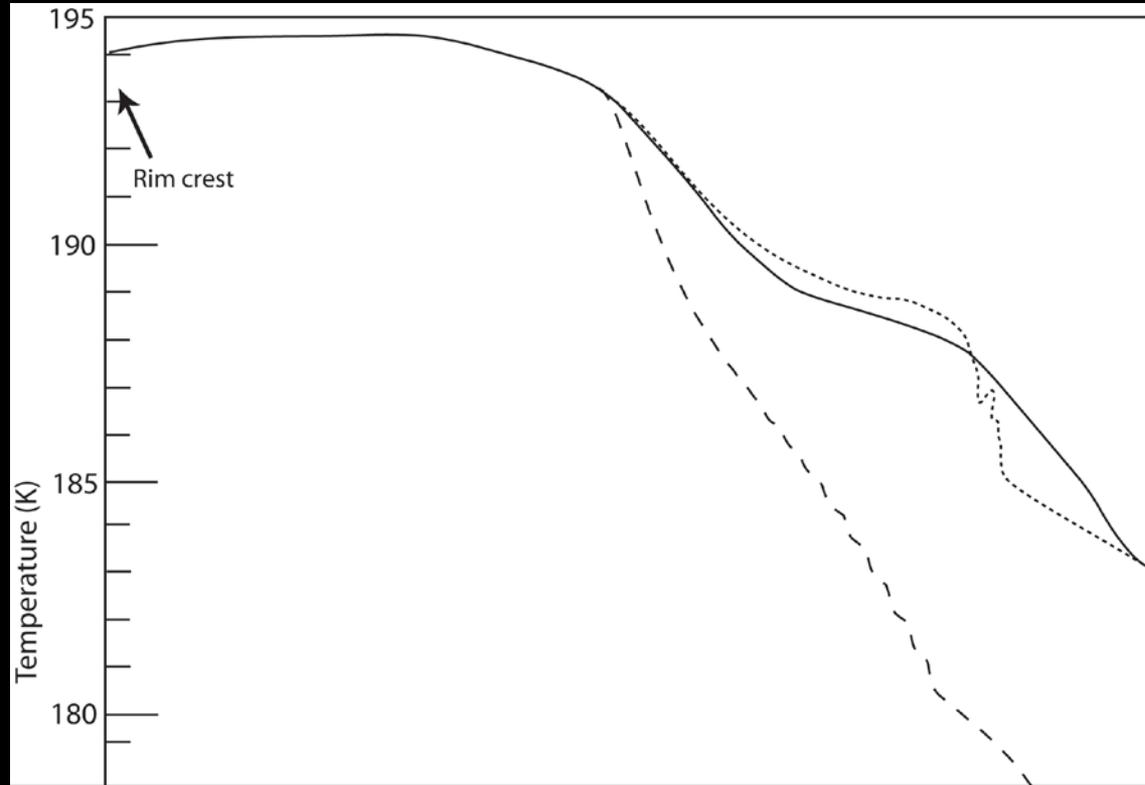
Plot of the observed infrared temperature (solid line), the surface convective temperature for a  $Ra_{eq} = 45$  (dotted line) and the surface convective temperature for a  $Ra_{eq} = 1000$  (dashed line)
