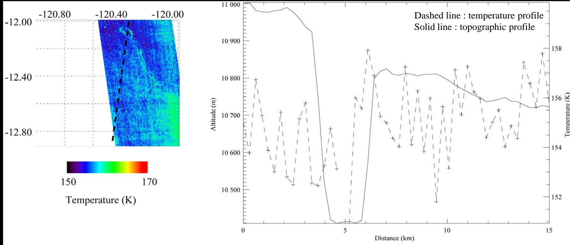
Geometry of the sinuous rille > Length : 36.5 km, depth : 520 m, wide  $\approx$  3 km
