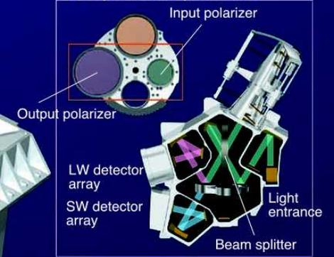
IRC (Near- & Mid-Infrared Cameras/Spectrometers)
