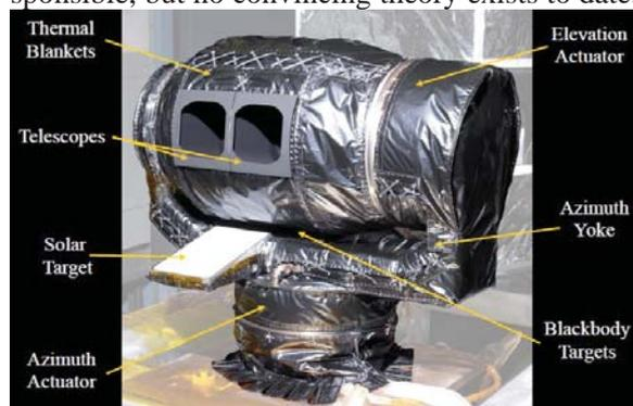
Fig. 1: The MRO/MCS flight instrument during thermal vacuum testing at JPL.
