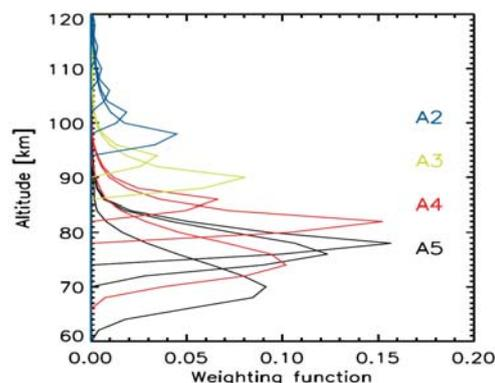
Fig. 2: Vertical response functions of a combined limb/nadir VCS temperature measurement from 500 km altitude. Colors indicate different channels covering the 15  $\mu\text{m}$  CO<sub>2</sub> band.
