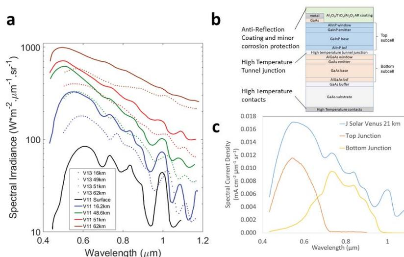
Fig. 1. (a) Solar spectra of the downward scattered solar radiation measured by the Venera 11 and Venera 13 descent probes. (b) Simplified cross-section schematic of a GaInP/GaAs 2J solar cell designed for Venus solar and high temperature operation. (c) Balanced spectral current density ( $\sim 2.25 \text{ mA cm}^{-2} \text{ sr}^{-1}$  for both junctions) for a 21 km/300°C Venus optimized solar cell using the measured 300°C EQE weighted by the 21 km Venus solar spectrum.
