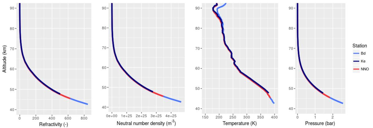
Figure 1: Refractivity, neutral number density, temperature and pressure profiles of the 2012.04.29 session. The profiles corresponding to the 32-m Badary (Bd) and 12-m Katherine (Ke) were derived from the open loop Doppler data obtained with the PRIDE setup, and the profiles of the 35-m NNO were derived using the frequency residuals obtained from ESA's PSA, corresponding to close loop Doppler tracking data.
