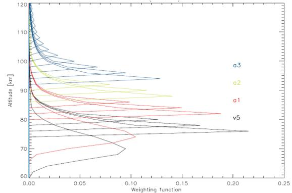
Fig. 2: Vertical response functions of a combined limb/nadir VCS temperature measurement. Colors indicate different channels covering the 15  $\mu\text{m}$  CO<sub>2</sub> band.
