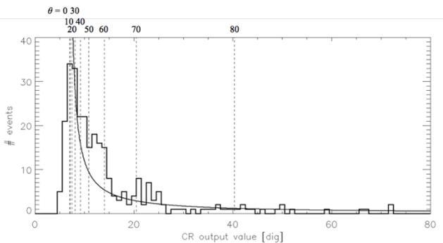
**Fig 1:** Cosmic-ray event distribution in the maximum recorded signal levels. The solid line shows the expected event number assuming the particle isotropic incidence, and the vertical dashed lines show the representative incidence angle in a interval of 10 degree.
