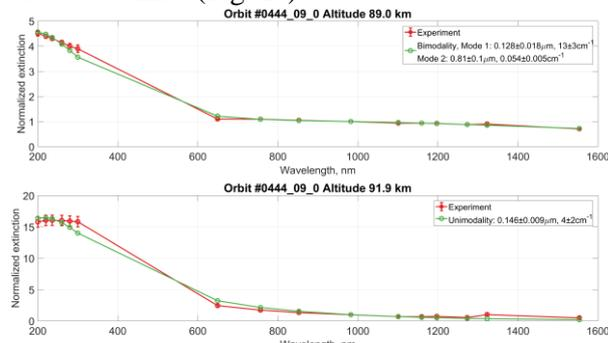
Fig. 1. Examples of fitted spectral dependence of aerosol extinction at altitudes 89 and 92 km of orbit #444.
