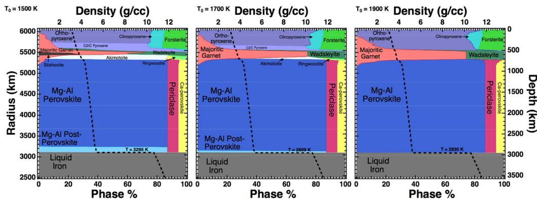
Figure 1: Planetary phase diagrams calculated by ExoPlex for a Venus-size planet of solar composition. Models are calculated using mantle potential temperatures of 1500 (left), 1700 (middle) and 1900 K (right). Density as a function of depth is shown as a dashed black line.
