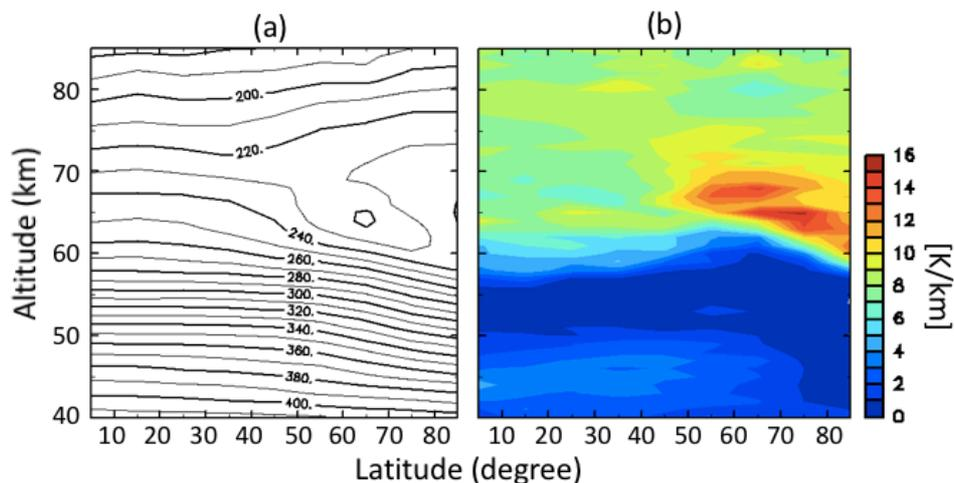
Latitude-height distributions of the zonally and temporally averaged (a) temperature and (b) static stability obtained by Venus Express and Akatsuki radio occultation measurements.
