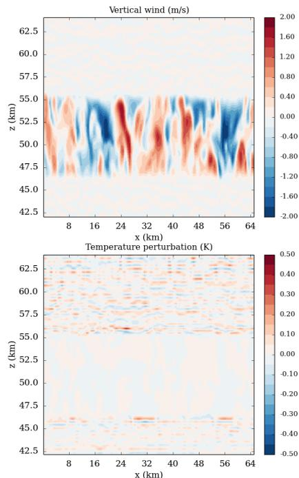
Figure 1: Top : vertical cross-section of the vertical wind (m/s). Bottom : vertical cross-section of temperature perturbation (K).
