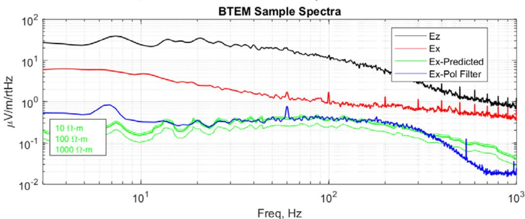
**Figure 2:** Analysis of 1 minute of data at float altitude 33 km. Large vertical (black) electric field is the primary and small horizontal (red) electric field is the secondary. Polarization filter drastically reduced coherent noise from air-traffic control transponder on the balloon avionics (blue). Predicted signal (green) using nominal quiet-day ionosphere is constant with ground resistivity 10-100  $\Omega$ -m.
