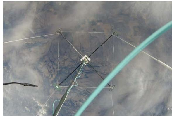
**Fig. 1.** BTEM in flight near Butte, MT, USA. Electric fields are measured between boom-tip electrodes (4-m separation); magnetometers are inside booms. Payload is spatially and electrically isolated from balloon avionics (teal cable in foreground is fiber-optic connector).
