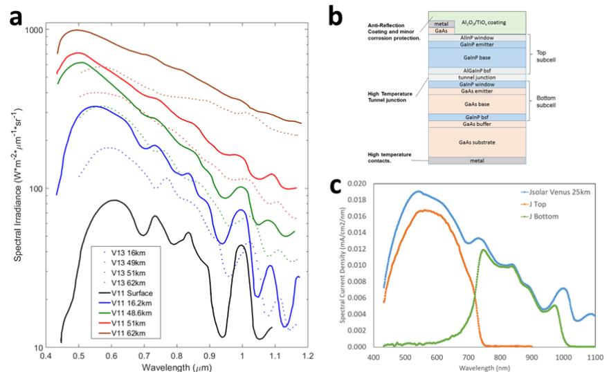
Fig. 1. (a) Solar spectra of the downward scattered solar radiation measured by the Venera 11 and Venera 13 descent probes. (b) Simplified cross-section schematic of a GaInP/GaAs 2J solar cell designed for Venus solar and high temperature operation. Calculated current density in the GaInP (3.90 mA/cm<sup>2</sup>) and GaAs (2.42 mA/cm<sup>2</sup>) subcells for the 300°C EQE data using the Venus solar spectrum at 25 km altitude where temperature is 300°C.
