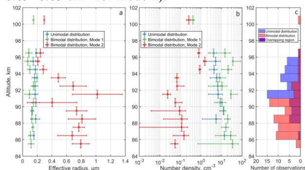
Fig. 2. Profiles of  $r_{\text{eff}}$  (a) and  $n$  (b) for unimodal and bimodal cases. (c) Altitude distribution of all observations.
