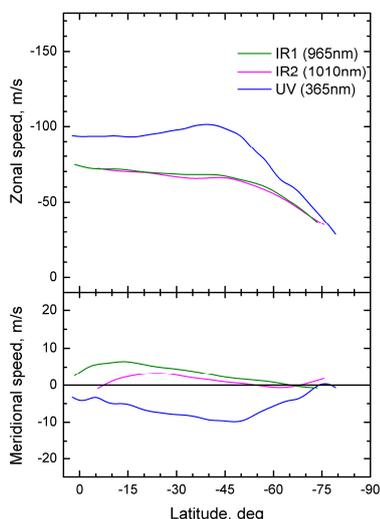
**Fig.1** Mean zonal (top) and meridional (bottom) wind latitudinal profiles, UV (blue, [3]), IR 965 nm (green, this work) and IR 1010 nm (magenta, this work).
