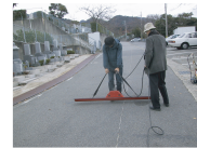
Fig. 5. Photograph showing the measurement way of 35MHz antenna across the Uzugamori fault (Site 2).
