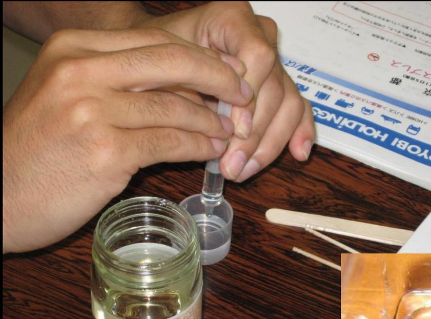
Silicon colloidal polish to get a smooth surface and to avoid any carbon-related contamination.
