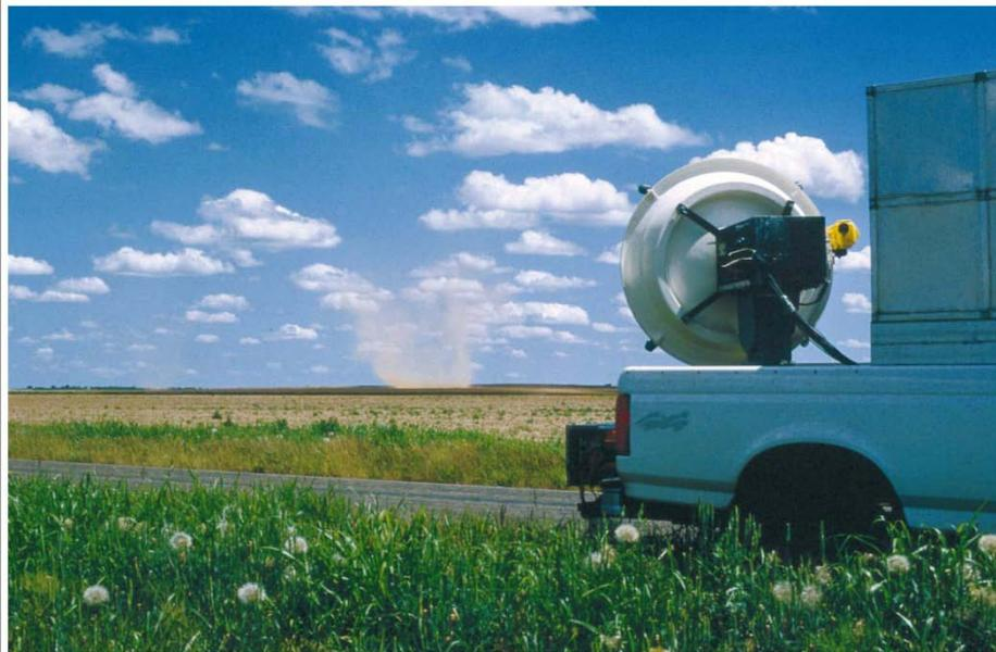
FIG. 1. Photograph of a dust devil just west of Tell, TX, on 25 May 1999, looking to the south-southeast, between 1514 and 1522 CDT. The antenna of the University of Massachusetts W-band radar, which is mounted on a pickup truck, is seen scanning the dust devil, which is moving away from the radar. The yellow structure mounted just to the right of the antenna is the boresighted video camera. Note the scattered cumulus clouds above the dust devil. (Photograph copyright H. Bluestein)
