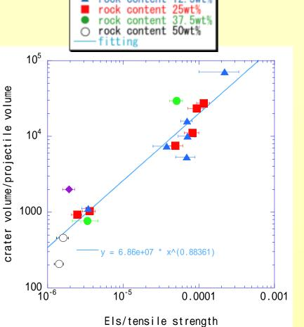
Fig.4 late-stage effective energy/ tensile strength versus Crater volume V/projectile volume  $V_p$
