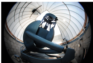
Figure 1: 0.81-m telescope at Tenagra observatory. The pixel scale and the field of view are ~0.87"/pix and 14.8 X 14.8 arc minutes, respectively.
