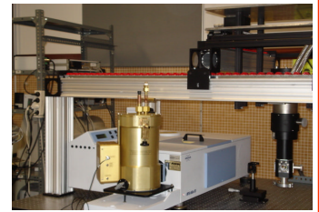
The spectrometer Bruker IFS 66vS, the movable cold finger and the bolometer
